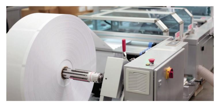
Bell and Howell's Inveloper® in action at AccuDoc Solution's headquarters in Morrisville, NC. The Inveloper® is one of the most efficient and productive mail finishing equipment available. It is designed to create envelopes on-demand using wrapping technology.
